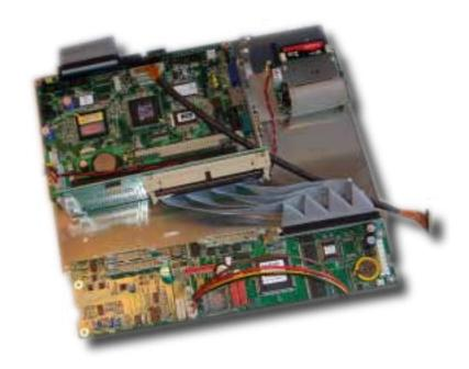
The SA-G142 is a CPU Upgrade Kit to upgrade the CPU from 6135 up to 6742 for SKIPPER GDS101 Navigational Echo Sounder Colour Screen Version.
